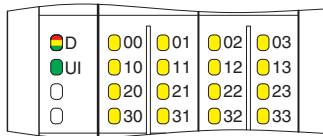
Fig. 4 Local status and diagnostic indicators
